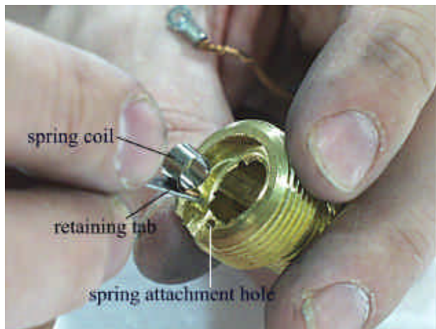
Figure 17: Close-up of Spring Coil and Retaining Tab
