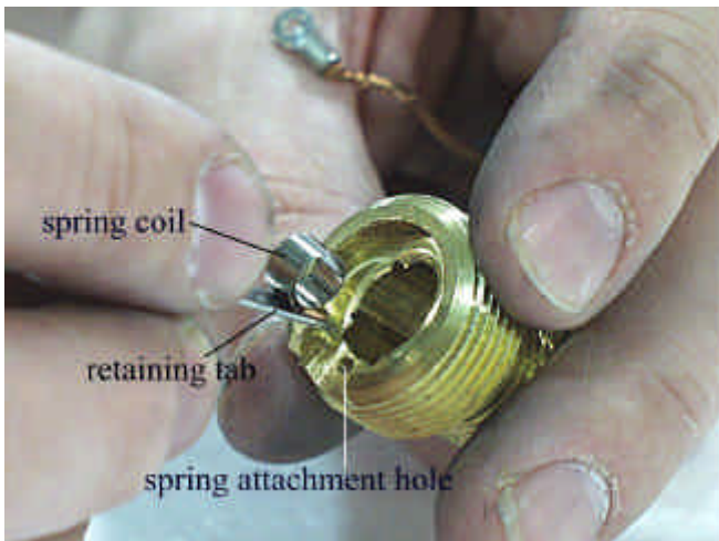
Figure 11: Close-up of Spring Coil (reference only)
