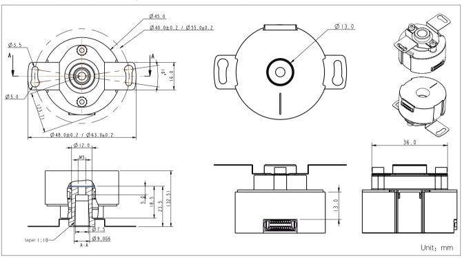
Hollow shaft (Ø6 or Ø8) with mounting hole diameter Ø46 tether)
