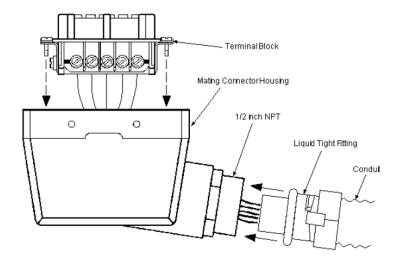
Insert wiring through liquid tight flexible seal and mating connector housing. Leave enough wire exposed to comfortably reach the terminal block. Wire to terminal block according to wire code in general instructions.
